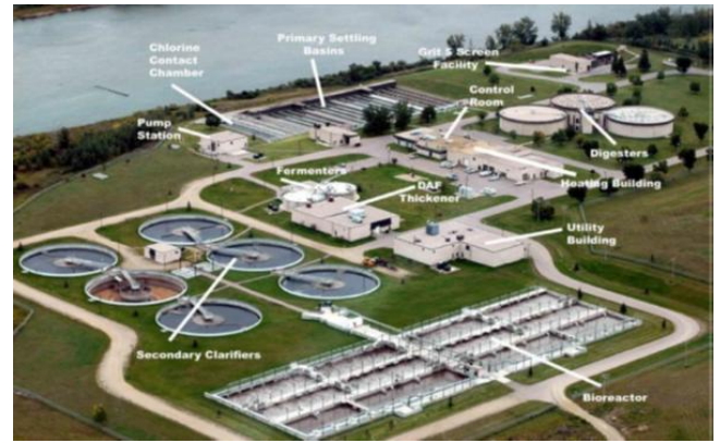
Fig.1 Wastewater treatment station model
