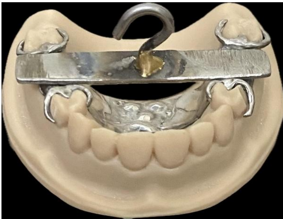
Figure 4: Metal plate attached to the geometric center of the framework.
