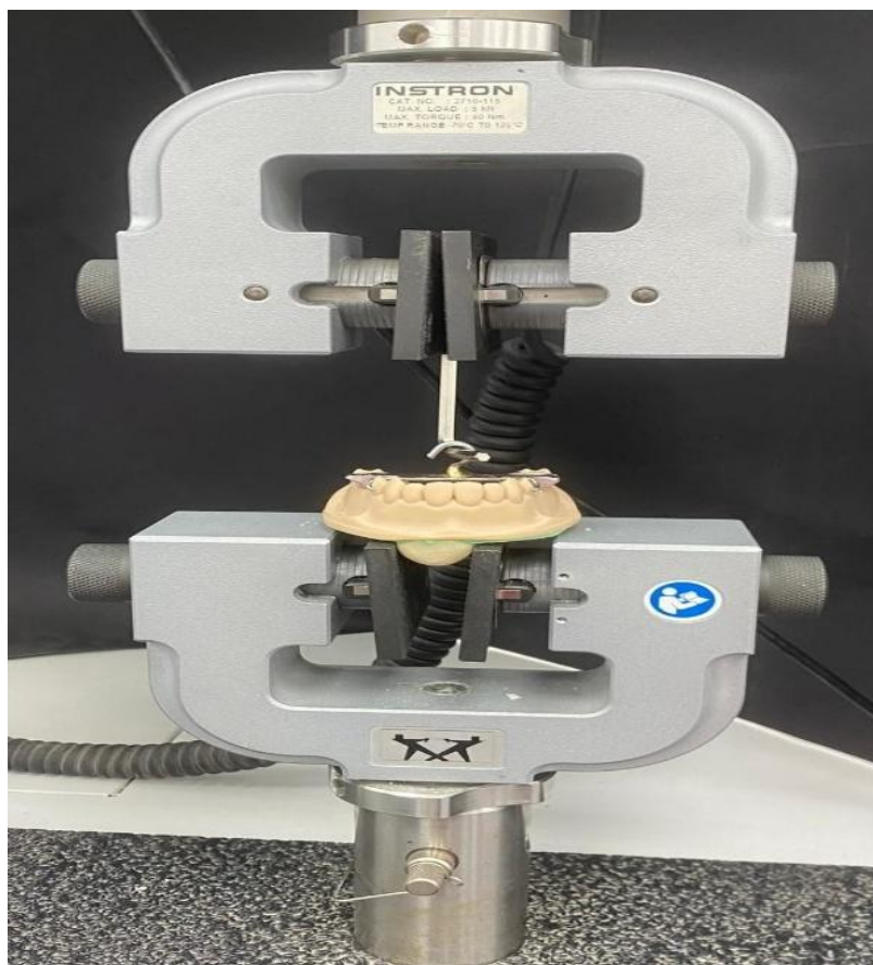
Figure 5: The framework attached to the Universal testing machine.
