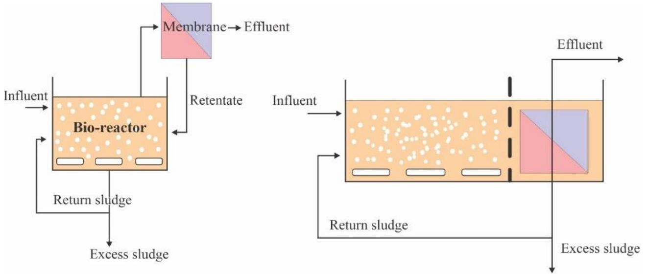
Figure 7. Membrane bioreactor (Conceived from Andersen et al.) [96]
