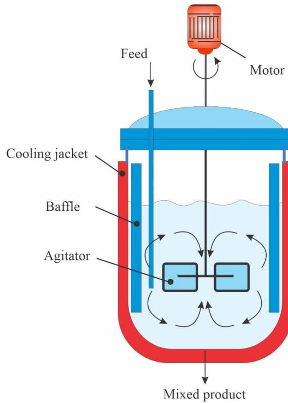
**Figure 1.** Continuous stirred tank fermenter (Adapted from Tavoosi et al.) [91]
