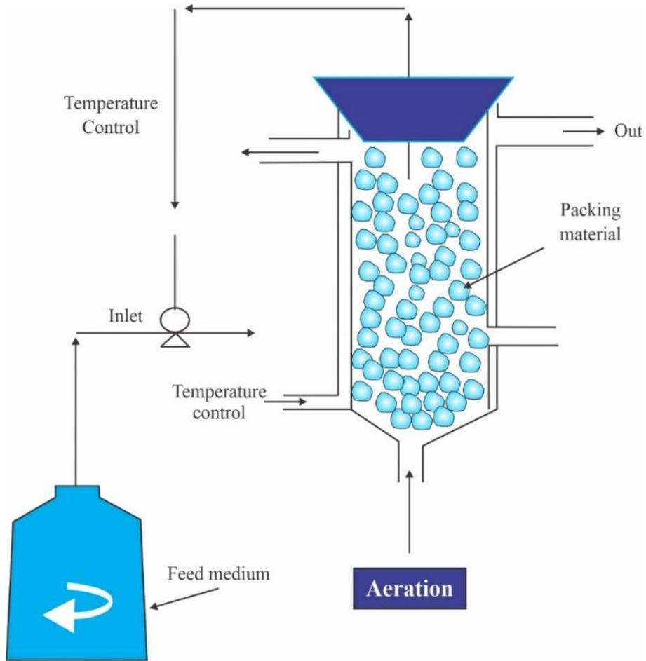
Figure 5. Packed bed fermenter (Adapted from Siegel and Robinson) [92]
