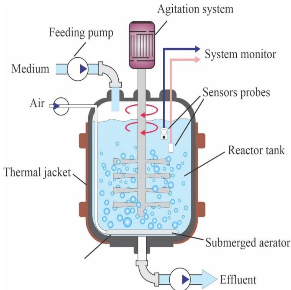
**Figure 9.** Continuous stirred tank bioreactor (Adapted from Saran et al.) [98]
