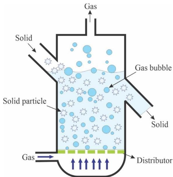
**Figure 4.** Fluidized-bed fermenter (Adapted from Kowng) [94]
