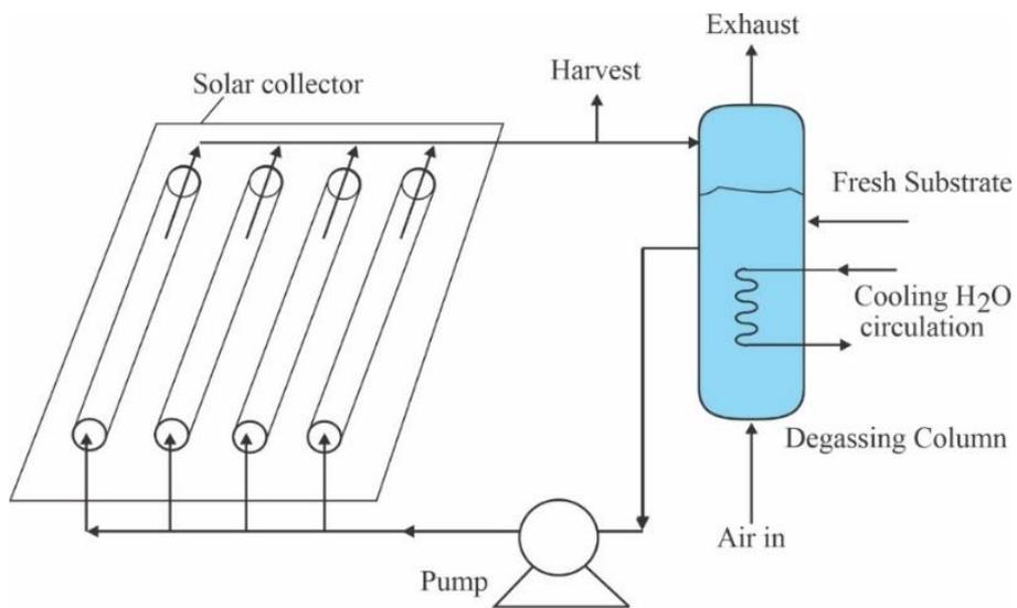
Figure 6. Photobioreactor (Redrawn from Sinha et al.) [95]
