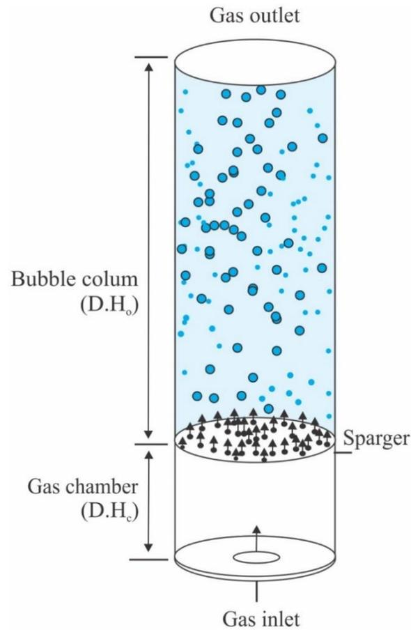
**Figure 3.** Bubble column fermenter (Adapted from Wilkinson et al.) [93]
