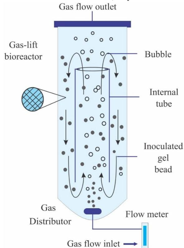
**Figure 2.** Airlift fermenter (Adapted from Siegel and Robinson) [92]
