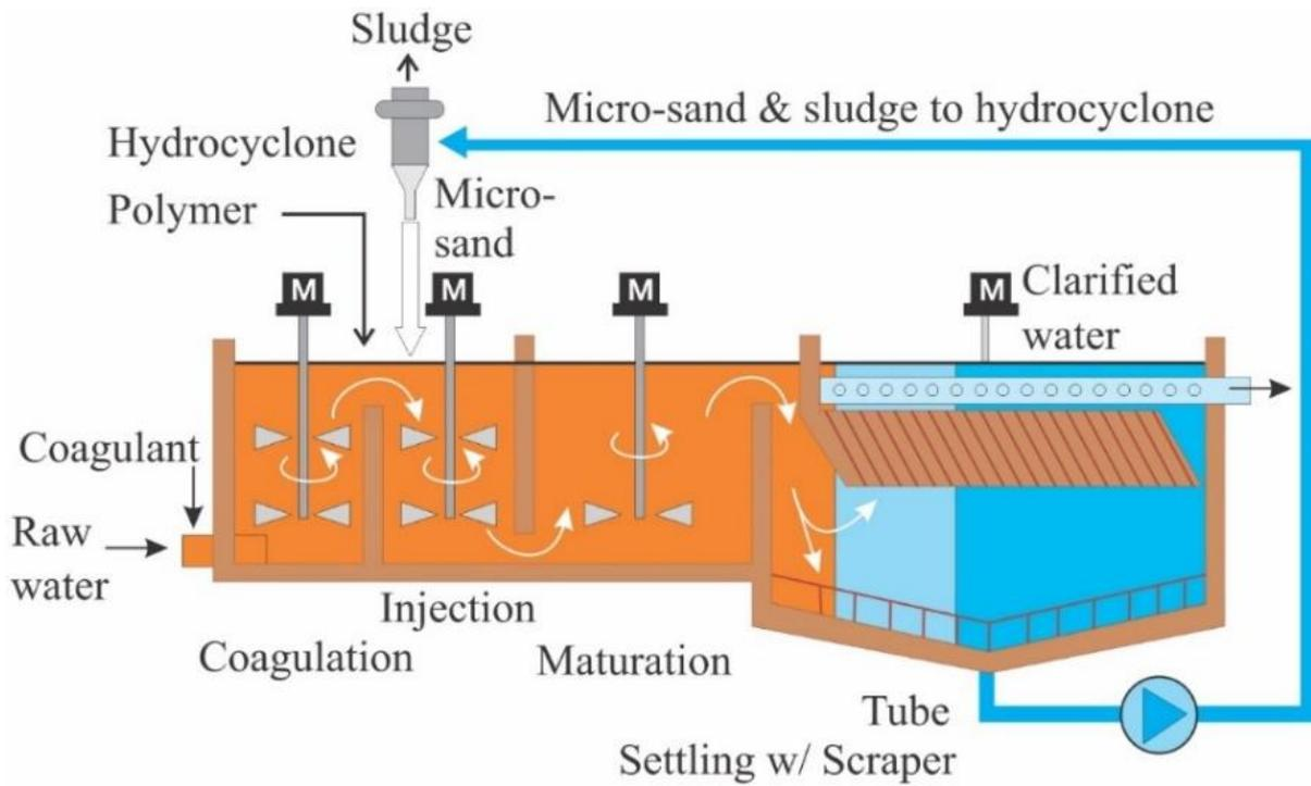
Figure 8. Ballasted floc bioreactor (Redrawn from Krüger published in Capodaglio) [97]
