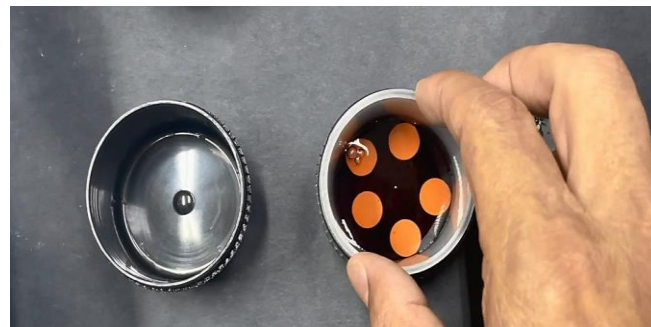
Figure 3: A; Disk-shaped specimens [ 2 mm×10 mm ] fabricated from monolithic zirconia blocks – B; Sample placed using acrylic resin in the center of the polypropylene holder.
