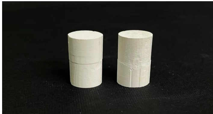
Figure 1: Monolithic Zirconia blocks milled from zirconia blank
