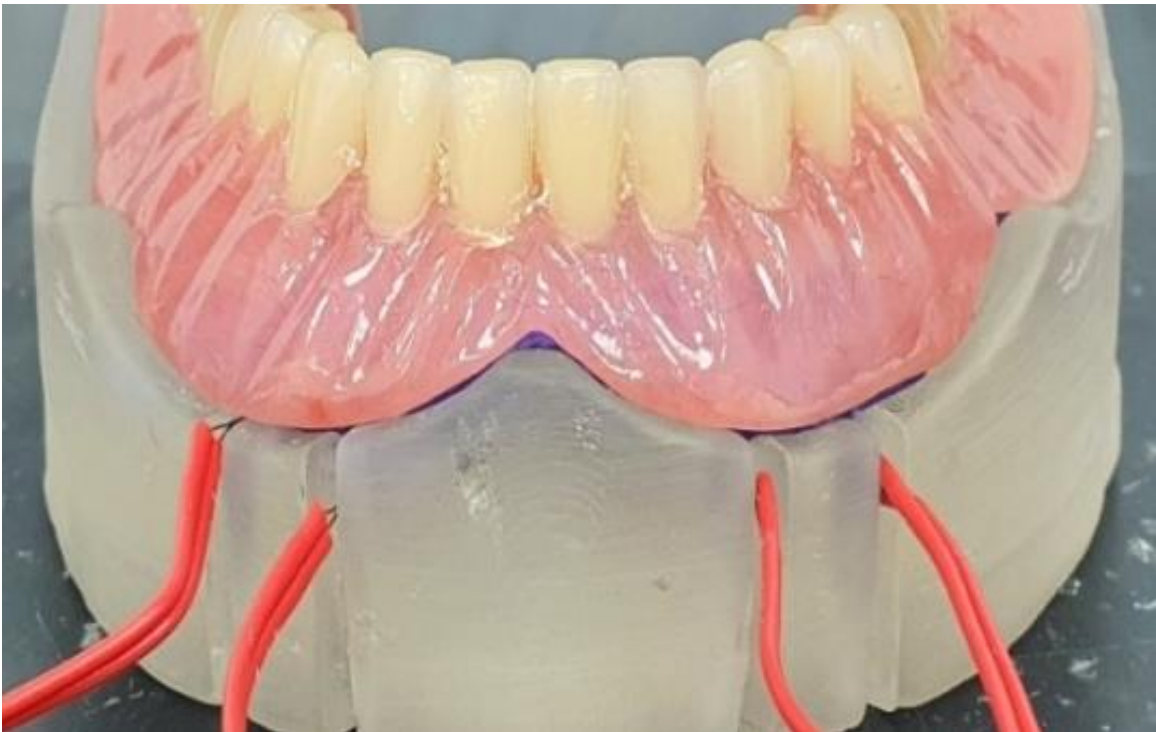
Figure 6 (b). Seated overdenture with connected strain gauges
