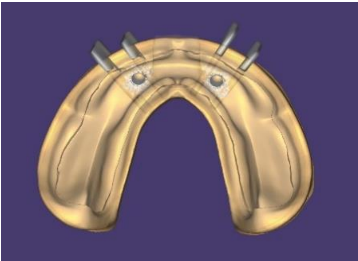
Figure 1(b). The two grooves for strain gauges
