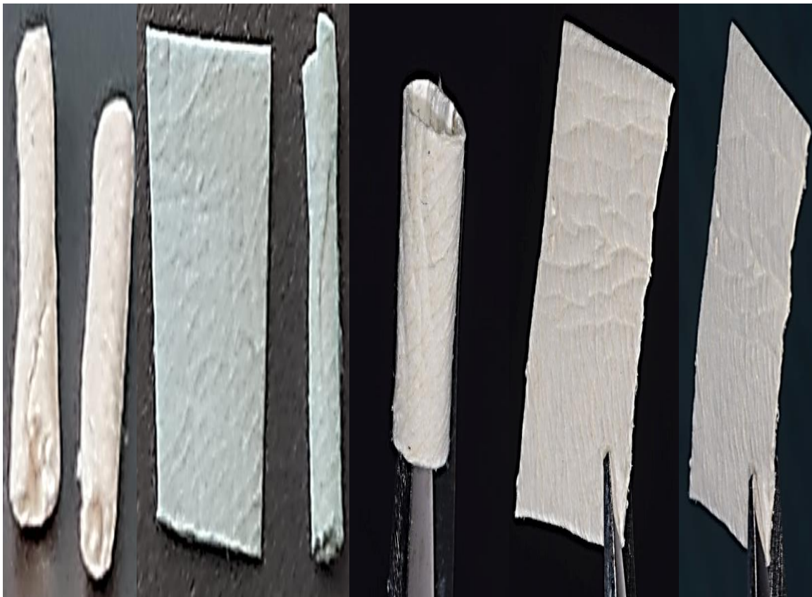
Figure 2: Fabricated PLA nanofiber scaffold.
